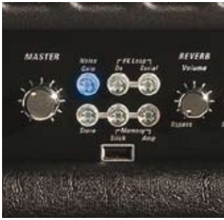
The usb port saves personal settings and uploads new sounds
